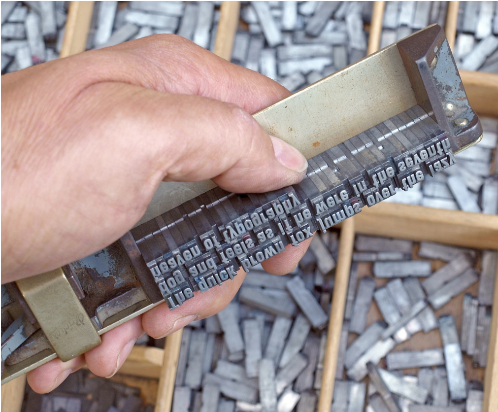
Left: A compositor makes up lines of text one letter at a time using a stick to hold them.
